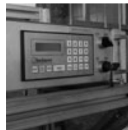
Tightness test to a pressure of 5 bar and 100 bar for bar tubes
